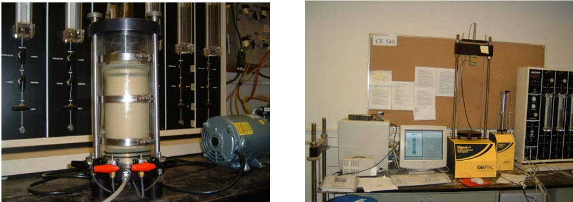
Figure 1. Set for Triaxial Experiment: a) Testing Chamber and b) Loading Frame
